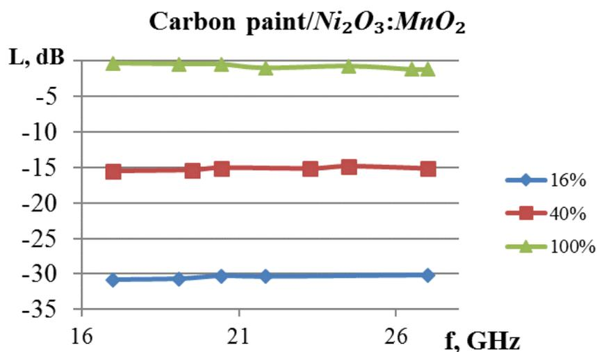
**Fig. 2.** Effects of the amount of oxide mixture on electromagnetic characteristics of composite
