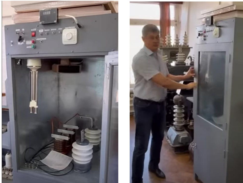
Fig. 2. High-voltage test chamber with the experimental setup.
