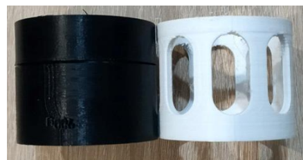
Figure 1 – Examples of nozzles for standard coils on the left and custom nozzle on the right
