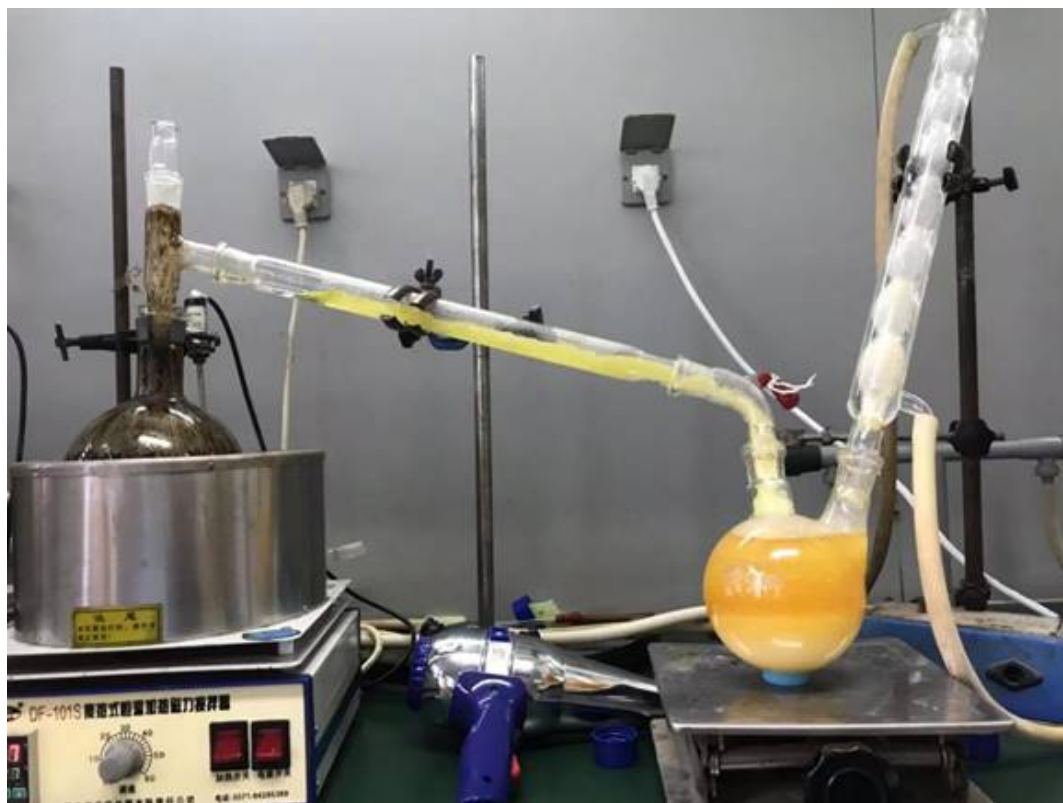
Figure 2.2 - Oligomer cleavage into rings
