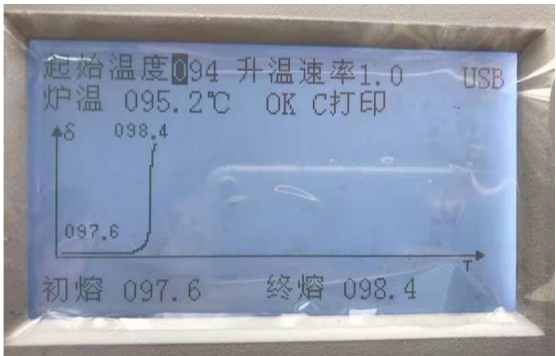
Figure 2.6 - Melting point of lactide measured by melting point tester
