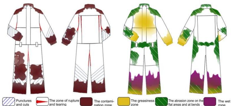
**Fig. 8. The topography of the influence of dangerous and harmful factors during the emergency and rescue operations in aviation:**
