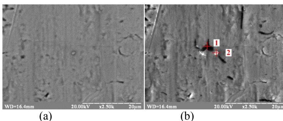
**Fig. 4.** The surface of titanium after electrochemical treatment, washing for 5 hours and immersion in a solution of an iron salt and lead (II) complex with PGMG. SEM images in the reflected (a) and secondary (b) electrons with an analysis of the chemical composition at the points:
