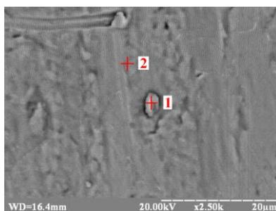
**Fig. 3.** The surface of titanium after electrochemical treatment and immersion in a solution of lead (II) complex with PGMG. SEM images with the analysis of the chemical composition at the points: 1. 94.12% Ti (IV) + 5.88% Pb (II); 2. 100% Ti (IV).
