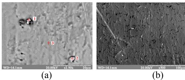
**Fig. 2.** The surface of titanium after electrochemical treatment and successive immersion in solutions of iron salts and lead (II) complex with PGMG. SEM images in the reflected (a) and secondary (b) electrons with the analysis of chemical composition at the points: 1. 49.90% Ti (IV) + 49.99% Fe (II) + 0.11% Pb (IV); 2. 70.29% Ti (IV) + 29.63% Fe (II) + 0.08% Pb (IV); 3. 100% Ti (IV).
