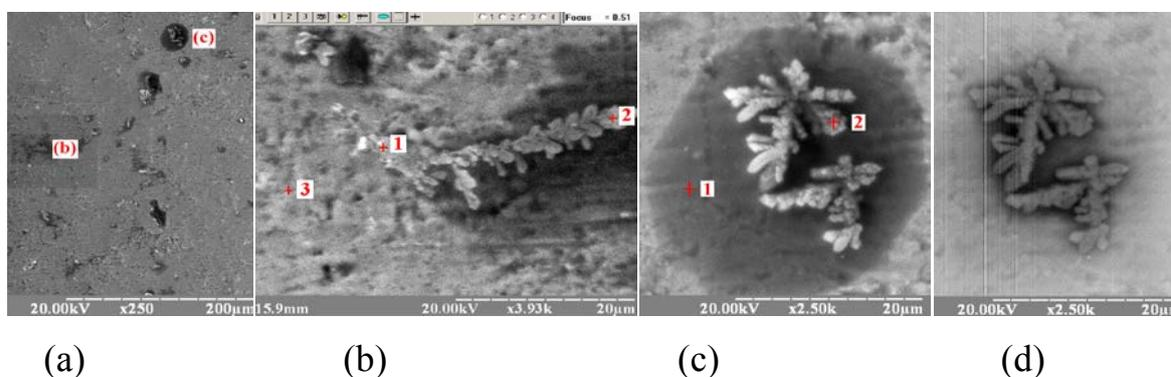
**Fig. 1.** The surface of titanium after electrochemical treatment in 6 M LiCl. SEM images in the secondary (a, b, c) and reflected (d) electrons with an analysis of the chemical composition at the points:
